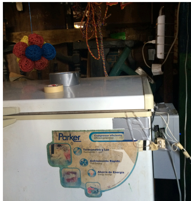
Image 1. The FlexBox in a Micro-Enterprise in Managua, Nicaragua. One can see the thermocouples inside the freezer, the box with the modem, microprocessor, modem, and telemetry, and in the back the switch controller that would be turned on and off at different times of the day depending on grid signals.
